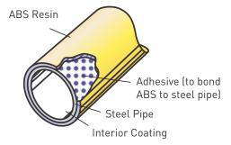
TECHNO pipe is steel pipe with ABS resin coated on the outer surface. An adhesive bonds the resin to the pipe preventing separation. The inner surface is treated with a non-corrosive coating.
